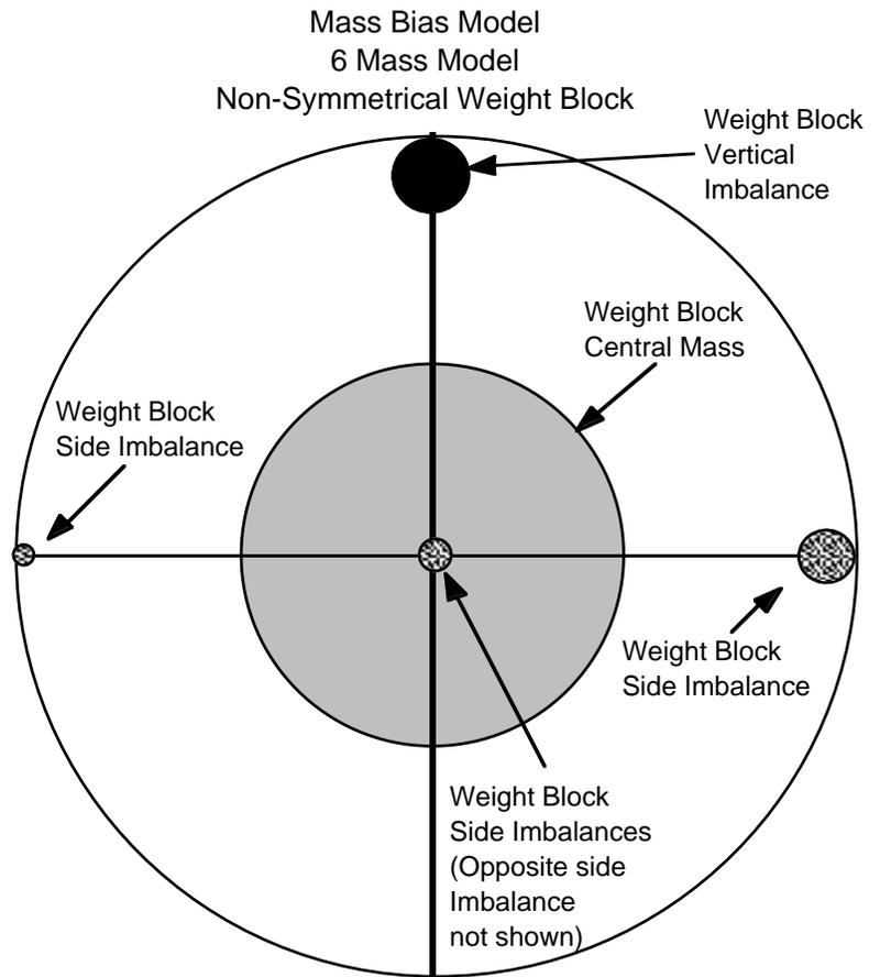
As the design of the weight block shifts the weight to the side, more mass bias is created. The model can then be changed to a 3 mass model. The center mass is still as before. The weight block vertical imbalance is as before. All of the sideways imbalance is modelled at one side. You will be able to see this effect in real weight blocks where the weight block very preferentially shaped in one direction.
