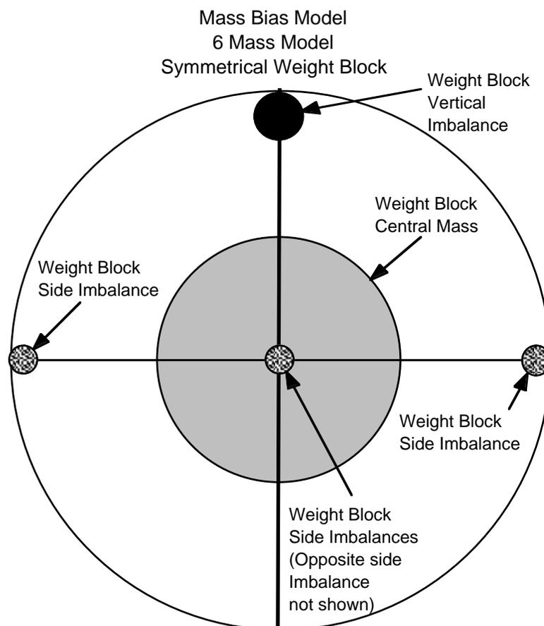
When the weight block is designed with more mass to one side, the mass distribution is changed. Since more mass is to one side the static balance is changed and the dynamic characteristics are also changed. The greater the “offset” mass to one side, the greater the mass bias.
