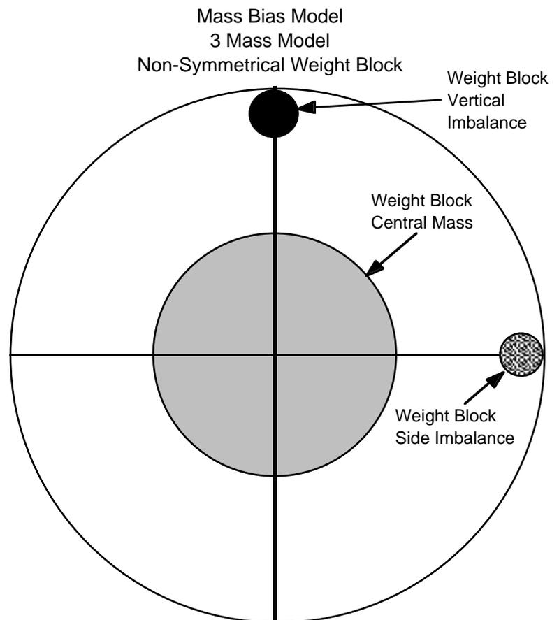
Shown below is a 3D model of a ball with a weight block that is designed with a large mass bias.
