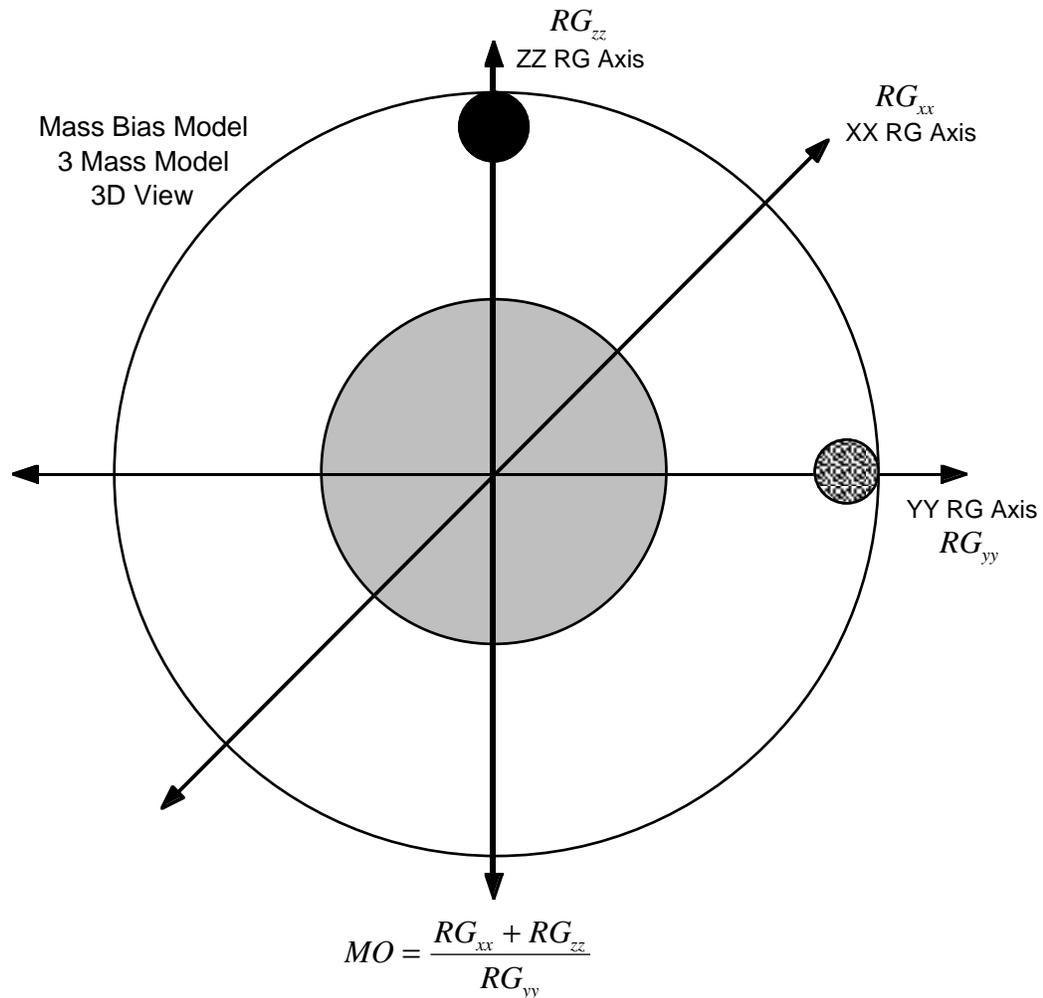
As the equation shows, the larger the values of RG measured about the XX axis and ZZ axis are and the smaller the value of RG measured about the YY axis is, the larger the MO Number is. And, since that's the way that mass bias is affected by different values of RG, the MO Number is related to the actual mass bias effect that the weight block has.
