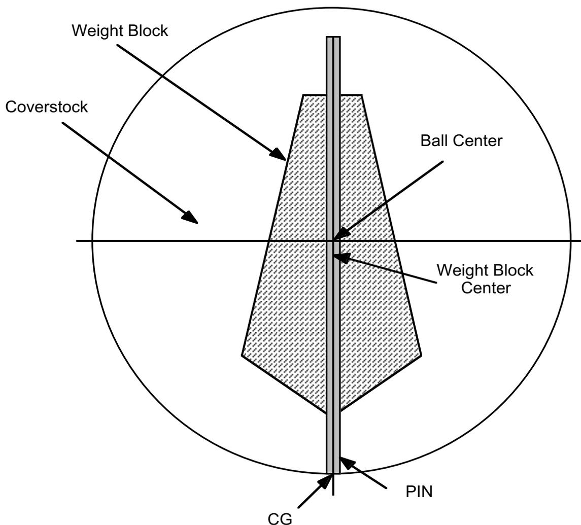
Another orientation that is still a PIN-IN design is shown in the graphic below. Generally, PIN-In balls focus their CG and PIN dynamic effects at the same time since the CG and PIN are at about the same physical location on the ball surface. Note that the ball weight block is rotated and shifted so the center of the ball is above and slightly to the left of the center of mass of the weight block.
